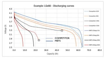
The MBTS system enables fast and precise thermal conditioning at all discharge rates (low and high). This leads to better and complete results even at extreme currents. Other systems have to stop operation  $(\circ)$  at high discharge rates due to thermal buildup, risking dangerous cell temperatures.
